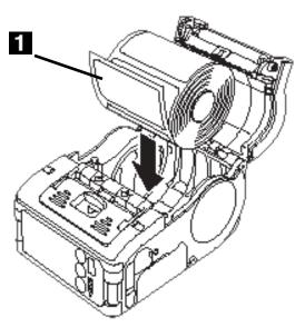
**Note:** When replacing a label roll of the same width as that used previously, adjustment of the label guide is not necessary.
